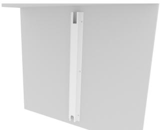
Metallic accessory for raising/lowering cables, joined directly onto the panel with screws. It houses the wiring in the space left when joining it to the panel. Dimensions: 712 x 121 x 76 mm. Finish: white, textured aluminium or titanium.
