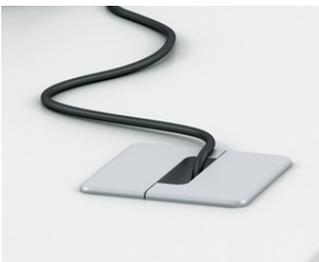
Made with two easy to assemble ABS plastic injection pieces. The interior diameter measures 80 mm; the exterior dimensions measure 94x94 mm. It has a gap to pass cables through. Available in several positions (view in price list).
