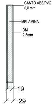
En PANELS: Acoustic screen manufactured in 19 mm melamine on high density with a sheet of 2.5 mm medium density fibreboard (MDF) on each surface, and upholstery with a felt of 0.8mm
