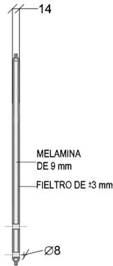
In PANELS: Composed of a 9 mm thick melamine board covered on each side with a felt of 3 mm thickness.
