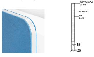
En PANELS: Acoustic screen manufactured in 19 mm melamine on high density with a sheet of 2.5 mm medium density fibreboard (MDF) on each surface, and upholstery with a felt of 0.8mm In REARS: Composed by a 2.5 mm DM sheet covered by one of its faces with the fabric.
